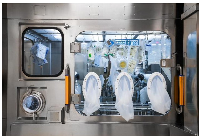
Fig. 3 – Steriline isolators guarantee the sterile environment for a safety packaging
